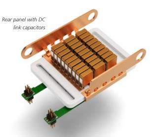
The design of the ceramic heatsink enables optimized heat dissipation of the SiC semiconductors on the upper side of the heat sink, while the DC link capacitor is integrated low-inductively in the power module on the underside of the heat sink via metallization that encompasses the cooler.
