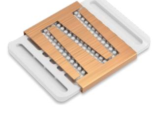
Another major advantage is that the pin-fin structure can be matched to the footprint of the SiC semiconductors in that there are the same number of cooling pins below the cooling lug. This allows optimum cooling of all chips.
